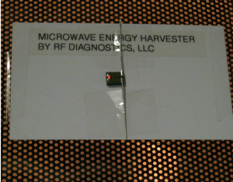
**Figure 3. Photo of the microwave oven energy scavenger using the RFD102A, red LED and a dipole antenna wires soldered to the module. The red LED lights up when the microwave is running.**
