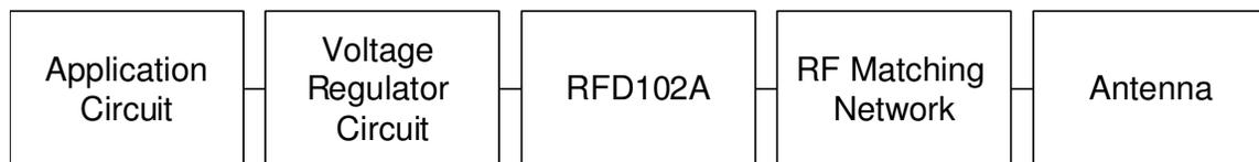
**Figure 2. Typical block diagram for a wireless energy harvesting system.**
