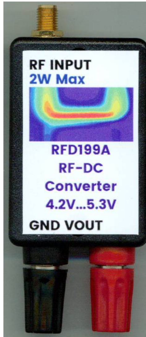
Figure 1. RFD199A photo. The plastic housing is 38.6mm x 57.6mm x 20.0mm and has an SMA connector at the RF input and two screw terminal banana plugs at the DC output.
